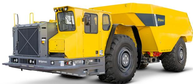
Fig. 1. The type of mine truck used for this study. The accelerometer is located centered on top of the rear wheel axis.
