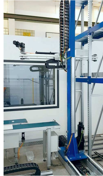
Fig. 2. Experimental testbed: stacker crane
