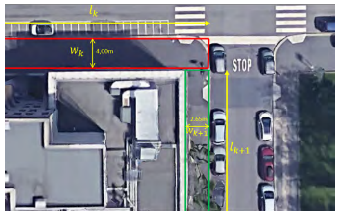
Fig. 2. Definition of the quantities of interest for the calculation of I_{width} .
