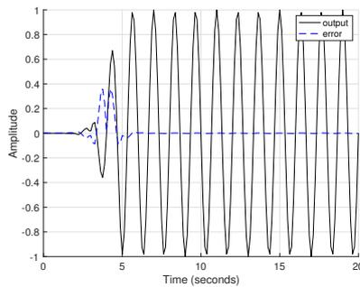
Fig. 3. System output tracking  $\sin(3\pi/2)t$  along with the delayed error
