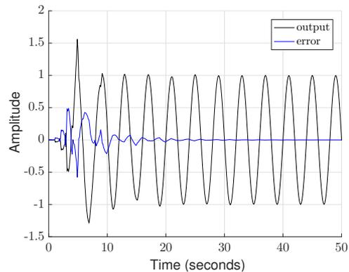
Fig. 12. System output tracking  $\sin(\pi/2)t$  under the additive perturbation  $0.3/(s + 1)$  to the plant
