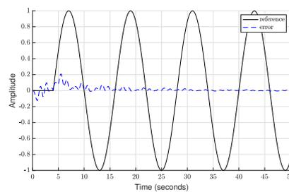
Fig. 9. Delayed error against  $\sin(\pi/6)t$  in the presence of the input disturbance  $\sin(3\pi/2)t$ .
