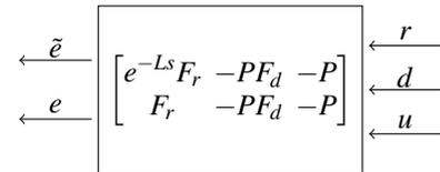
Fig. 8. Generalized plant in the presence of input disturbance  $\sin(3\pi/2)t$ . That is, the tracking frequency is below the Nyquist frequency while the disturbance above the Nyquist frequency enters into the plant input. We take the following weights:
