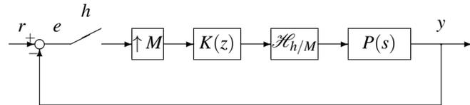
Fig. 1. Sampled-data feedback system
