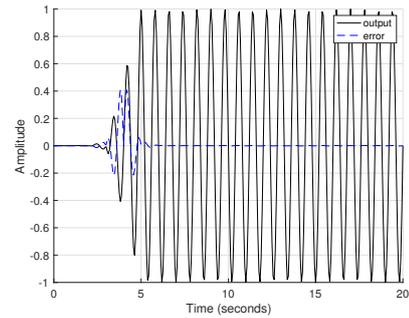
Fig. 6. System output tracking  $\sin(5\pi/2)t$  along with the delayed error
