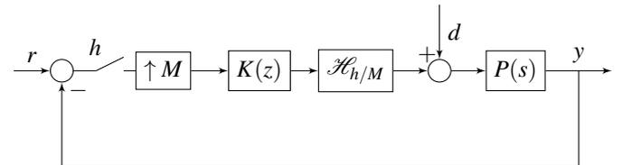
Fig. 7. Sampled-data feedback system with input disturbance
