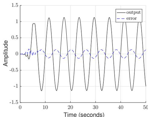
Fig. 11. System output tracking  $\sin(\pi/3)t$  under the additive perturbation  $0.05/(s + 1)$  to the plant
