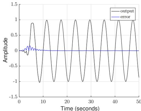
Fig. 10. System output tracking  $\sin(\pi/3)t$  without disturbance
