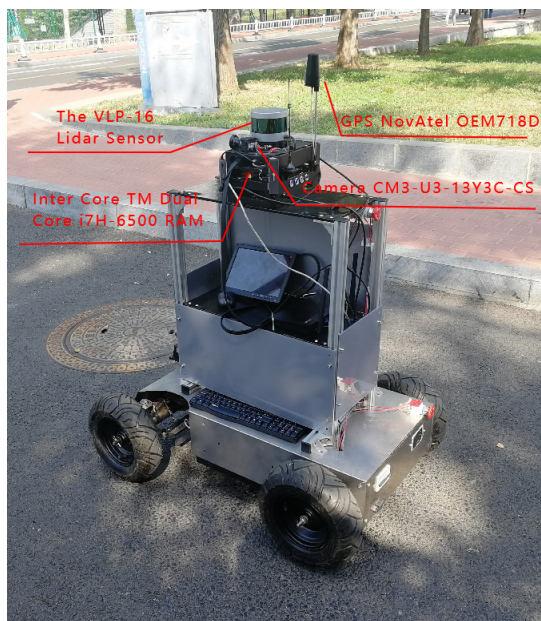
Fig. 6. The setup of the mobile robot equipped with a VLP-16 Lidar sensor. The computer is IPC(Industrial Personal Computer) (Intel Core TM Dual Core i7H-6500 and 6GB RAM) without the GPU, the GPS is NovAtel OEM718D.
