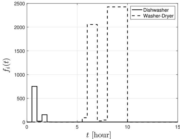
Fig. 3. Examples of two real loads in a house. Again, the loads are shifted for optimum visibility; otherwise, the user wants to schedule all at the beginning.
