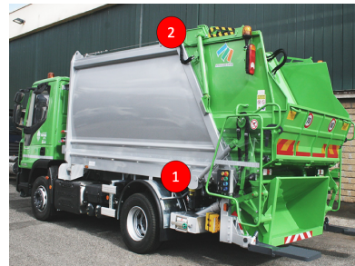
Fig. 1. Experimental setup. The red circles indicate the positions of the inertial sensors.
