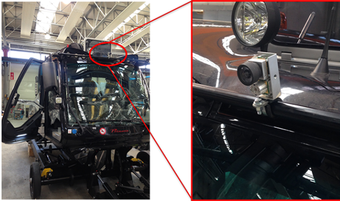
Fig. 1. Experimental Setup: Prinoth Leitwolf with the 2D LiDAR sensor mounted on the top of the cabin
