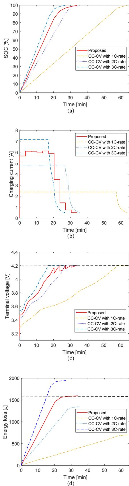
Fig. 3. Battery's responses of (a) SOC, (b) charging current, (c) terminal voltage, (d) energy loss.
