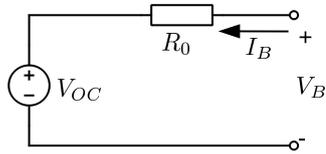
Fig. 1. Battery equivalent circuit model.
