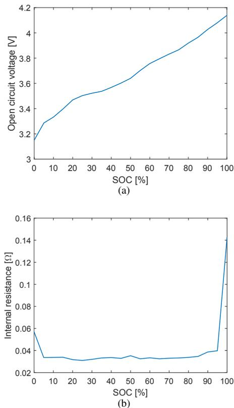
Fig. 2. Relationship between the battery’s (a) SOC and open circuit voltage, (b) SOC and internal resistance.
