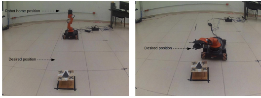
(a) The end-effector home position. (b) The desired position in the x , y and z directions for regulation control (static object).
