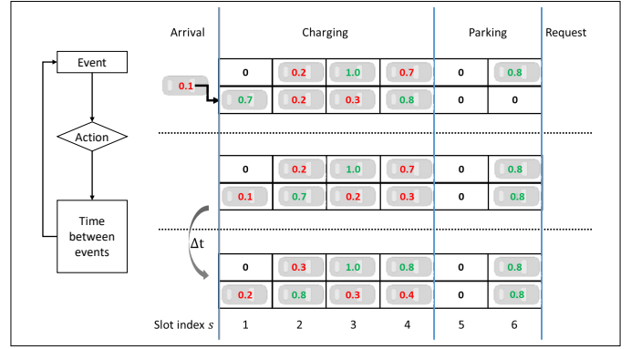
Fig. 3. Simulation framework: high-level flowchart (left) and example of a vehicle arrival event (right) showing the position and SOC of vehicles within the Park and Charge Lanes.
