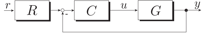
Fig. 2. The closed-loop system with a reference governor as shown in Fig. 2. From (8), one can expect that the reference governor designed as
