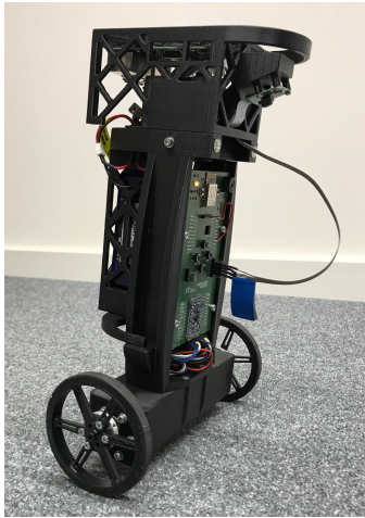
Fig. 9. EduBal equipped with a vision module consisting of a Raspberry Pi 3B and camera used in the task of following a line on the ground
