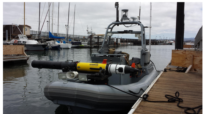
Fig. 1. A REMUS 100 autonomous underwater vehicle (AUV) on a SeaFox unmanned surface vessel (USV).
