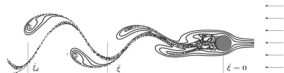
Fig. 1. Vortex shedding in the 2-D flow behind the cylinder (Aamo and Krstic, 2004)
