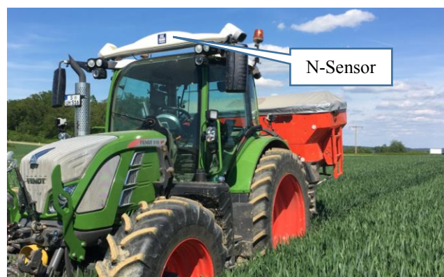
Fig. 1: Yara N-Sensor ALS2 mounted on the tractor roof.
