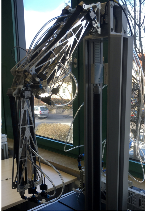
Fig. 1. Experimental setup of the robot actuated by pairs of pneumatic muscles. The three rotary degrees of freedom will later be denoted by \alpha_1 , \alpha_2 , and \alpha_3 . In the experimental setup, the three angles, as well as the pressures of the pneumatic muscles, pneumatic valves, and of the air supply are measured in order to apply the feedback controller.
