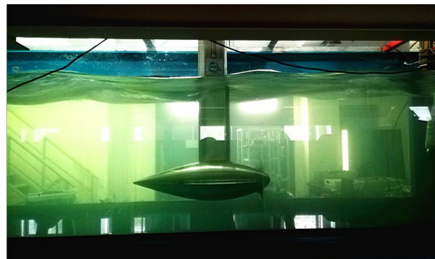
Fig. 7. Current tunnel with MCT and data acquisition system.
