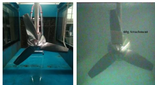
Fig. 8. Blade with rope to create a mass imbalance condition.
