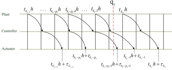
Fig. 2. Signal transmission around  $q_s$ .
