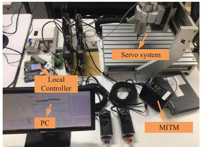
Fig. 5. Self-developed physical experimental platform
