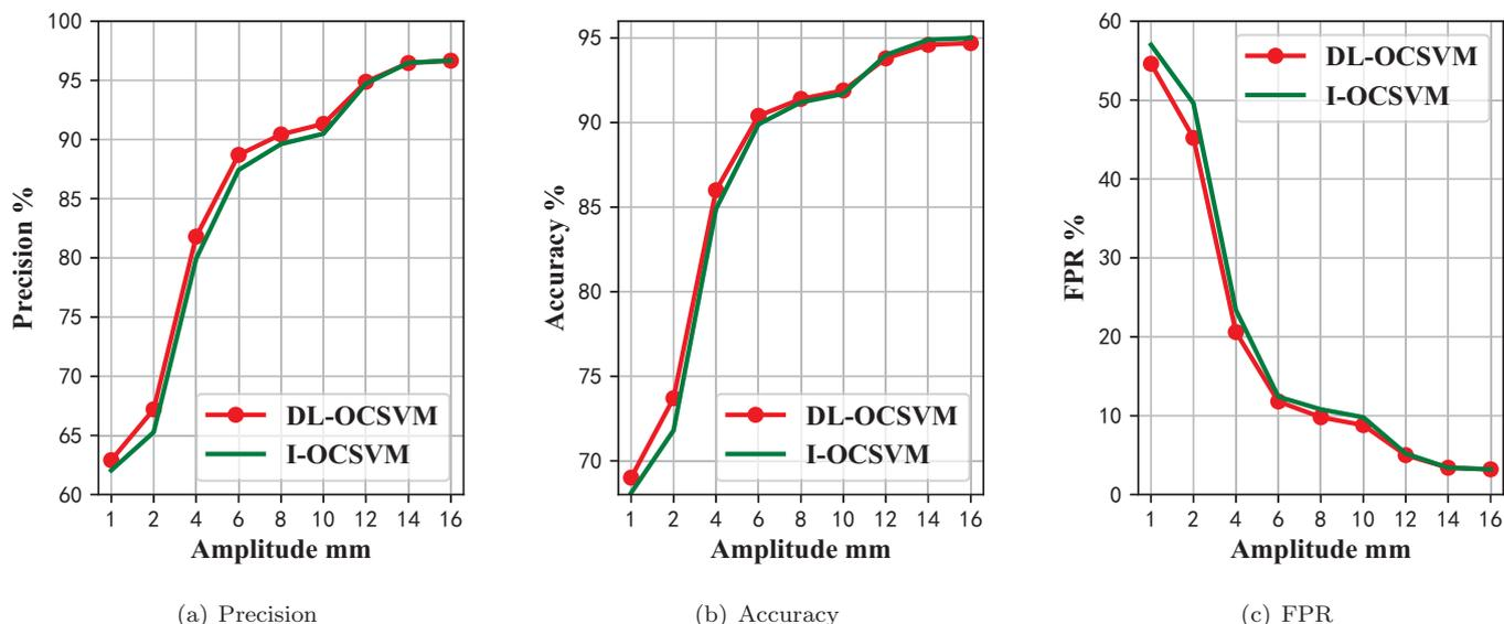
Fig. 7. Performance comparison between DL-OCSVM and I-OCSVM under different attack amplitudes
