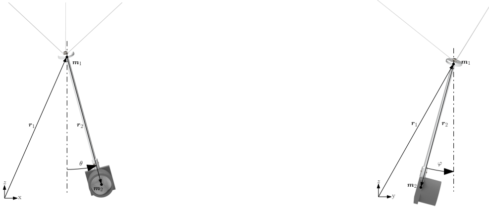
Fig. 3. x - z view (left) and y - z view (right) of spherical pendulum
