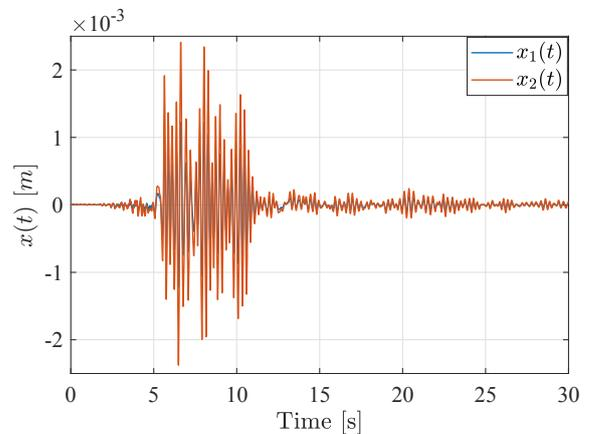
Fig. 5. Relative displacement of the building with input delay  $\tau = 0.4$ , plus time-delay compensation by multiple observers.
