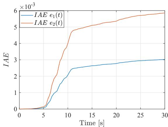
Fig. 6. IAE performance index of  $e(t)$  obtained with the closed-loop system (15) and (19) when  $\tau = 0.4$ .
