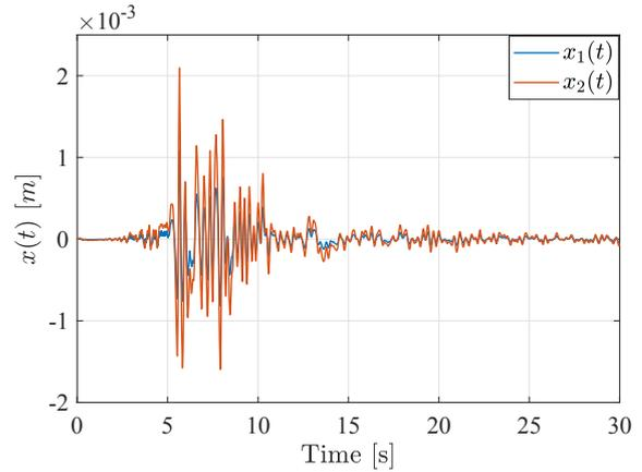
Fig. 4. Relative displacement of the building with input delay  $\tau = 0.1$ , plus time-delay compensation by a single observer.
