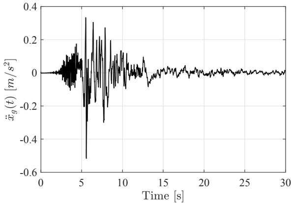
Fig. 2. The 1940 El Centro earthquake record.
