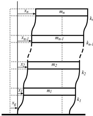
Fig. 1. Multi storey structure with  $n$ -degrees of freedom.
