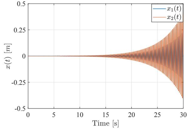
Fig. 3. Relative displacements of the building without time-delay compensation, here  $\tau = 0.1$ .
