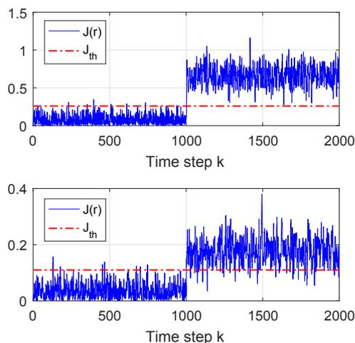
Fig. 3. FD results for the faulty case 1 and 2.
