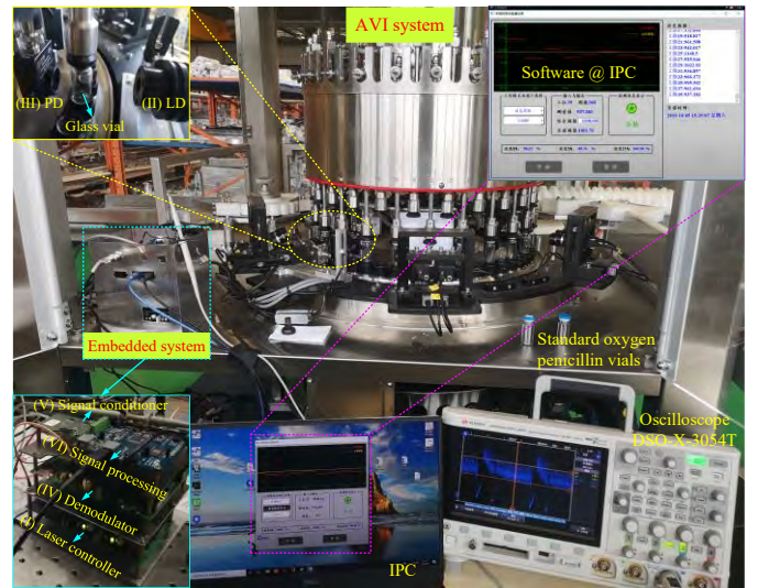
Fig. 2. The TDLAS/WMS prototype photo and testing scene, taken at the Truking Academician Workstation.
