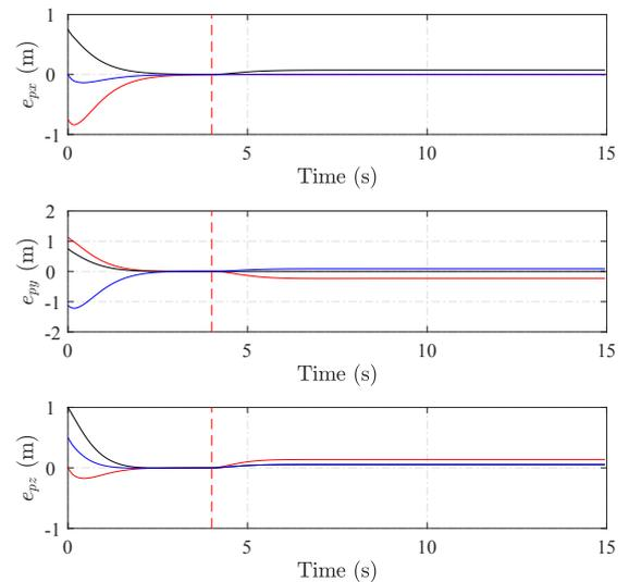
Fig. 4. Position tracking errors of quadrotor team using traditional optimal control policies.
