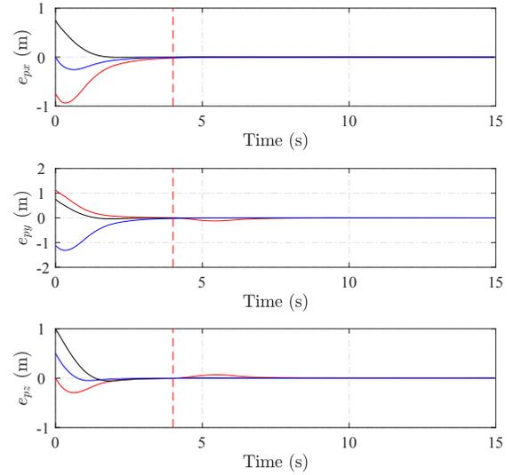
Fig. 3. Position tracking errors of quadrotor team using the proposed controller.
