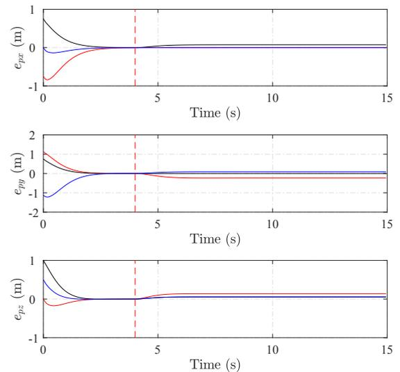
Fig. 4. Position tracking errors of quadrotor team using traditional optimal control policies.
