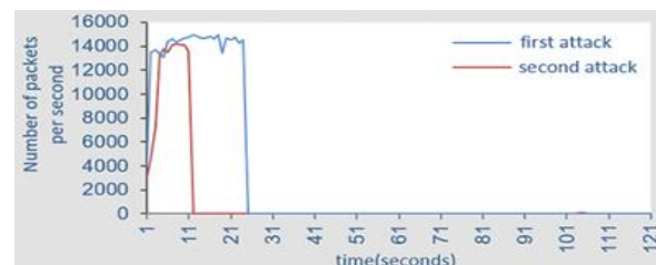
Fig.6. Number of reflected packets per second transmitted to the network by the IoT device and machines
