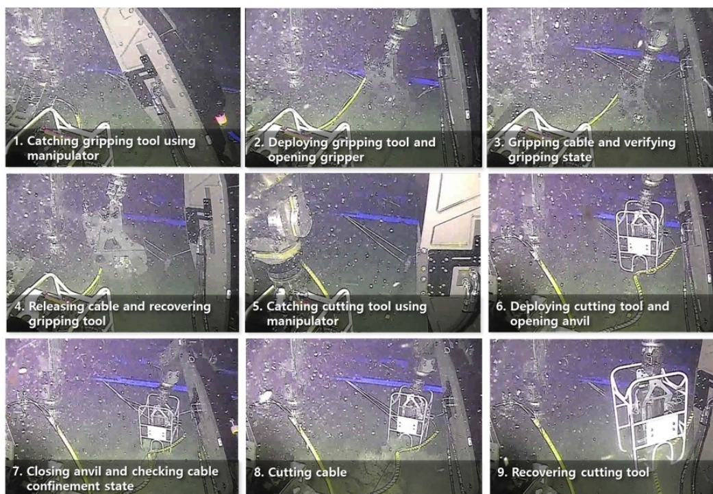
Fig. 14. Test for cable maintenance
