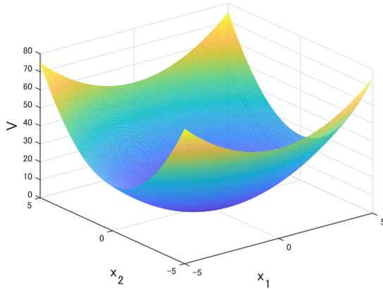
Fig. 2. Tracking Control Lyapunov Function:  $x_1 - x_2$
