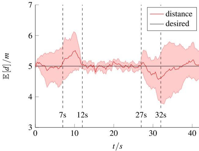
Fig. 2. Monte Carlo simulation showing mean and variance of distance trajectory with time varying power constraint.
