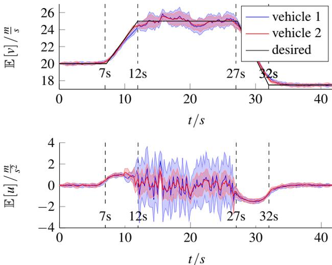
Fig. 4. Monte Carlo simulation showing mean (solid line) and variance (shaded area) of velocity/control inputs. Due to the higher importance of compensating the process noise in this scenario, the variance increases during the time interval in which the power constraint is active [12s:27s].
