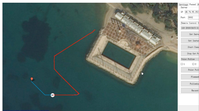
Fig. 8. Path following simulation: the blue line shows the remainder of the planned path generated with a modified A* algorithm (Wang and Xiang (2018)).
