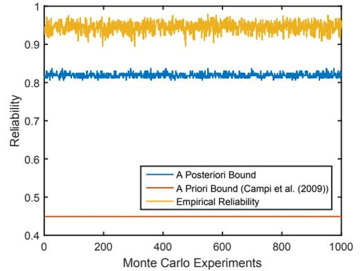
Fig. 2. The comparison of different guarantees of interval reliability under 1,000 Monte Carlo experiments
