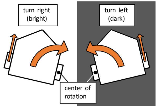
Fig. 3. Behavior rule of the mobile robot.
