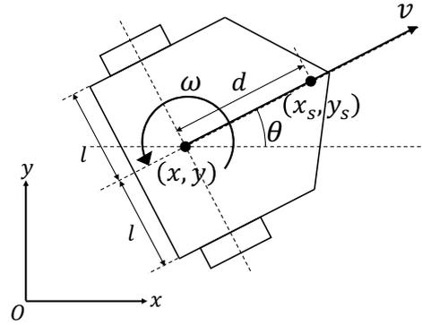
Fig. 2. Model of the mobile robot.
