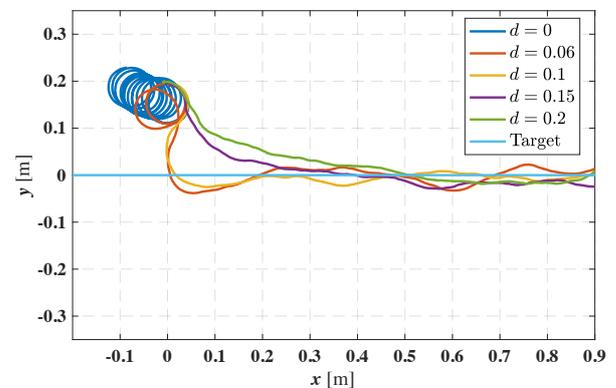
Fig. 15. Influence of the sensor position  $d$  on the resulting routes.
