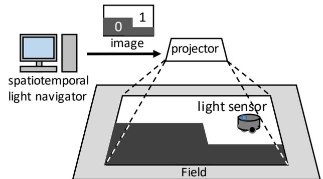
Fig. 1. Conceptual diagram of spatiotemporal light navigation system.
