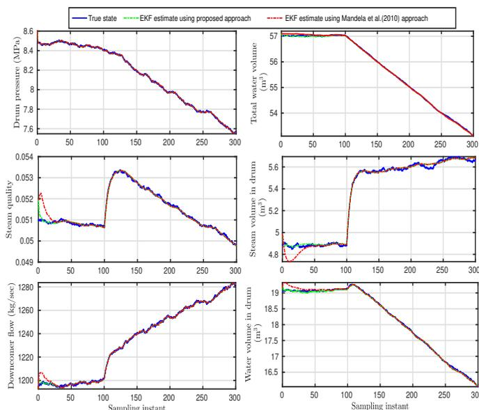
Fig. 3. State estimates: Drum boiler
