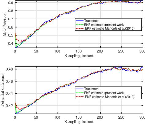
Fig. 1. State estimates: Galvanostatic charge process
