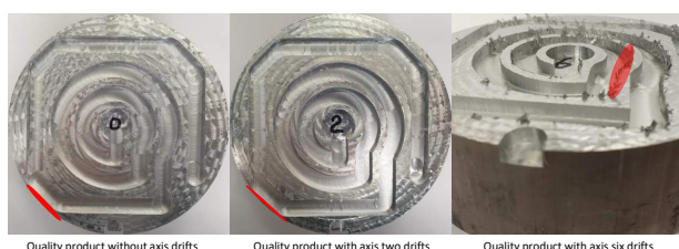
Fig. 5. Severity of the sixth axis deviation on product quality.
