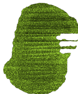
Fig. 7. Triangulation of the detected worn region points using alpha complex with \alpha = 0.9 .
