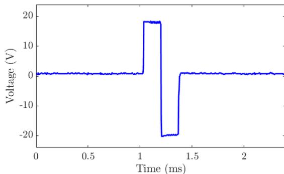
Fig. 1. A single stimulation wave, with a pulse width of approximately 135 microseconds.
