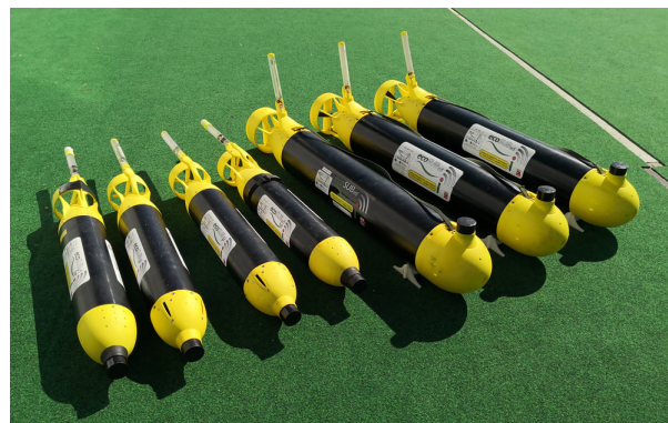
Fig. 1. The ecoSUB \mu 5 (first four on the left) and ecoSUBm5 (right) AUVs.
