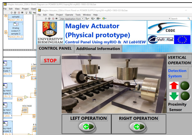
Fig.5. Developed human-machine interface using NI-LabVIEW software.
