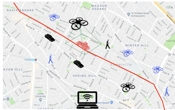
Fig. 1. Example of processing network : smart sensors (in blue and black) collect, process, and communicate data to track the state of a vehicle (in red) in the presence of communication and computation latency.
