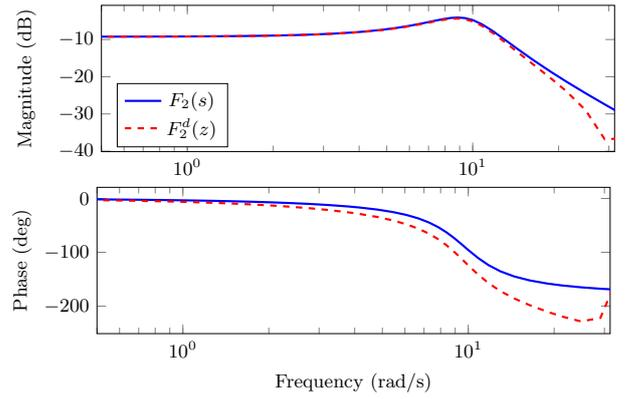
Fig. 1. Frequency Response of CT ( $F_2$ ) and DT ( $F_2^d$ ) Kautz BF's for slow sampling.
