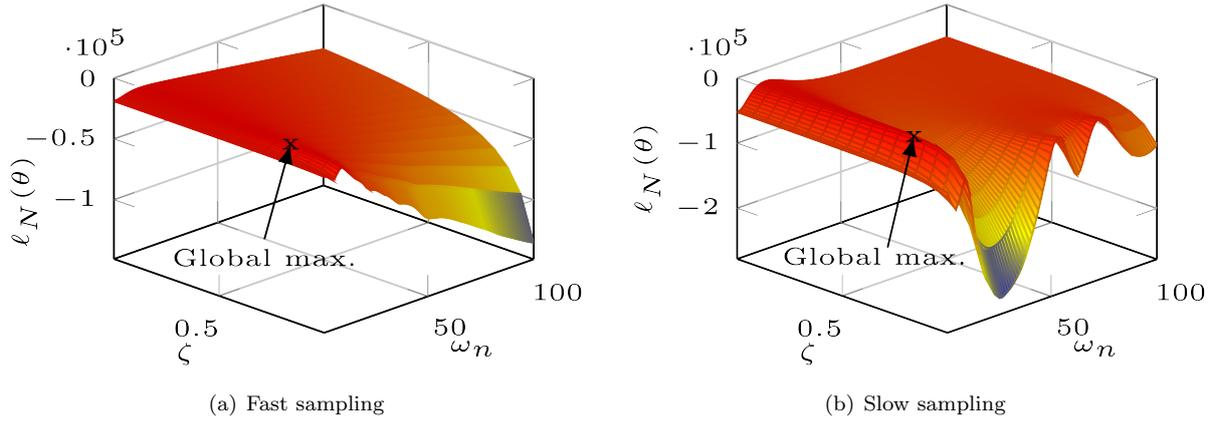
Fig. 2. Log-likelihood function for case known model structure. For (a) fast sampling and (b) slow sampling.
