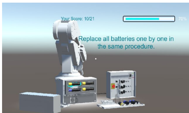
Fig. 2. Gamified training for changing robot arm battery with points, progress bar and signposting (Nguyen and Meixner (2019)).
