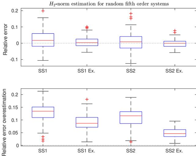
Fig. 3. RE and REO boxplots using first- and second-order stable-spline kernels for random fifth-order systems, 100 random systems, 100 measurements and additive white measurement noise with SNR 20. Ex. denotes that optimal input design was used to select the input sequence. The input sequences are limited as  $\mathbf{u}^T \mathbf{u} = 100$ . The boxes indicate the median and the 25th and 75th percentiles, the whiskers indicate the extreme values and + denotes outliers.
