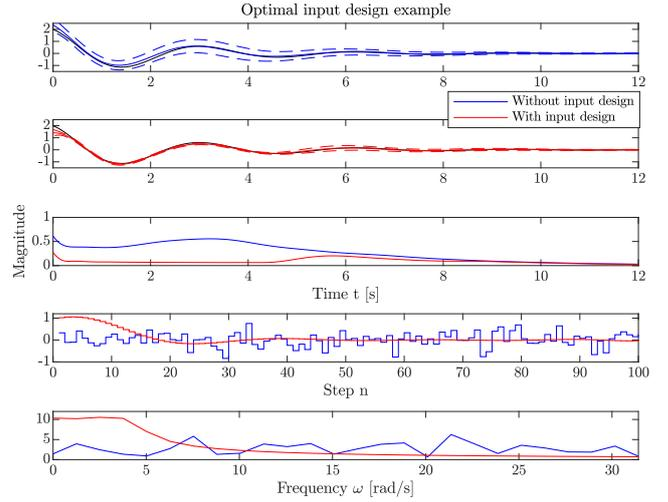
Fig. 2. Experiment design example on the system  $G(s) = \frac{2s}{s^2 + 0.8s + 4}$  using a second-order stable-spline kernel (4) with an oscillating component,  $\kappa(s,t) = \kappa_2(s,t)(\cos(\beta_2|s-t|) + 1)$ , as suggested in Chen (2018). 1: GP system identification for white noise input scaled to energy limit. 2: GP system identification for optimal input. 3. Comparison of  $3\sigma$  confidence bounds. 4: Input sequences in time domain. 5: Input sequences in frequency domain.
