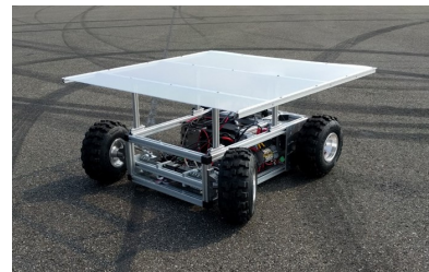
Fig. 1. The model-scale experimental UGV IRT-Buggy equipped with a landing platform measuring 1\text{m} \times 1\text{m}
