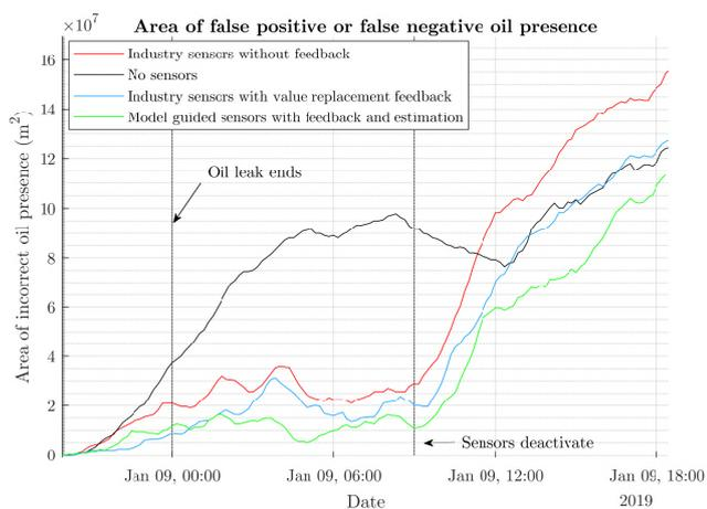
Fig. 3. A comparison of the oil presence error of the simulations. Note how all sensor approaches reduce error by 70% while sensors are active, with the model guided sensors being approximately 60% as erroneous as industry standard pathing and continuing to have less error after sensing stops.
