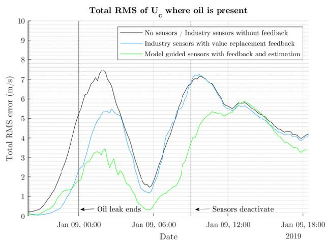
Fig. 4. A comparison of the RMS error of current flow velocity where oil is present. Note the 30% to 50% in reduction in error the model guided sensors with feedback and estimation displays over the industry sensors using value replacement, and the continuation of less error after sensing stops.
