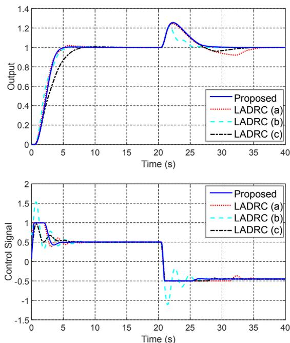
Fig. 2. System responses by using different methods
