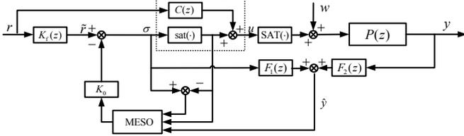
Fig. 1. Block diagram of the proposed control scheme
