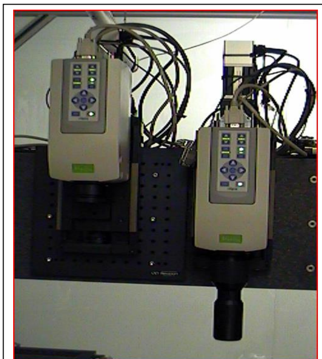
Fig. 1. Two Mid-Wavelength InfraRed cameras (Merlin Mid InSb MWIR) with the large field of view (left) and the small one (right) with resolution 7.57[ \mu\text{m}/\text{pixel} ]. Cameras can be moved vertically for changing fields of view and autofocusing.
