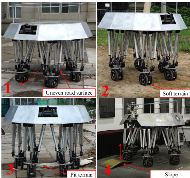
Fig. 6. Schematic diagram of attitude adjustment in different terrain.
