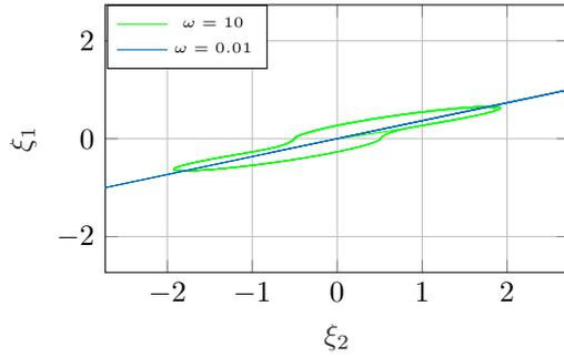
Fig. 4. State trajectory under sine input  $\phi = \sin(\omega t)$  for  $d = -0.5$ ,  $k_2 = b = 3$ ,  $k_1 = \frac{1}{3}(2\bar{k}_1^* + \bar{k}_1^*)$ .
