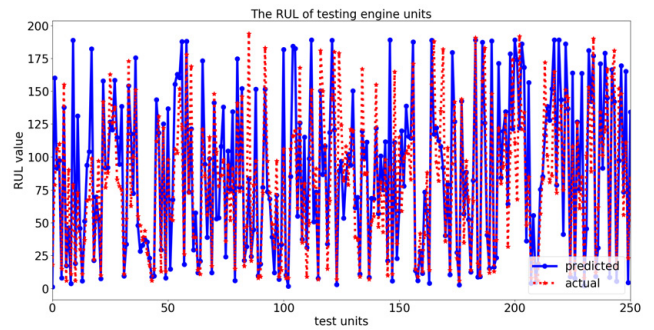
Fig. 8. RUL prediction for 250 testing engine units in FD002 subdataset
