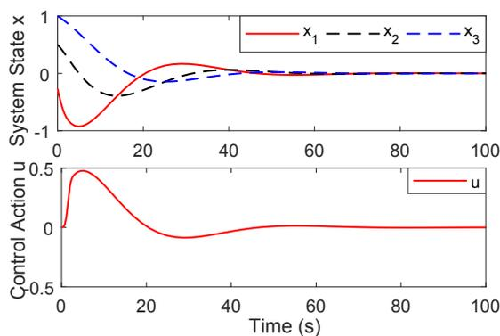
Fig. 3. The profile of controlled system states  $x$  and control  $u$ .
